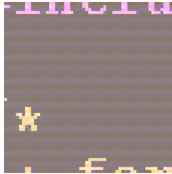
Figure 6: Artifact from the use of single-line processing. The horizontal streaks are a result of different line averages in a two-dimensionally designed dither pattern. This artifact can be avoided by using single-line dither.
