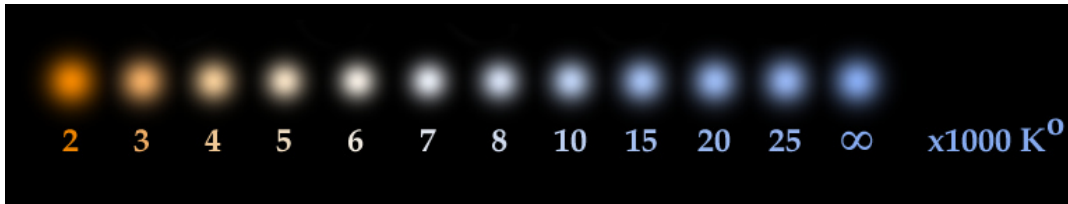
Figure 12. Rendered color scale using area variations to preserve brightness at different temperatures.
