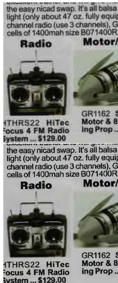
Figure 2. Comparison of JPEG at 100dpi (top) with quality factor 30% and DjVu (bottom). The file sizes for the complete pages are 82KB for JPEG and 67KB for DjVu
