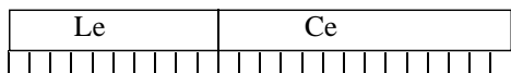
Figure 1. 24-bit encoding. L_e is the encoded log luminance, and C_e is the encoded uv color index.
