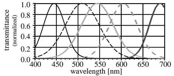
Figure 5. Spectral transmittances of optimal filter set.
