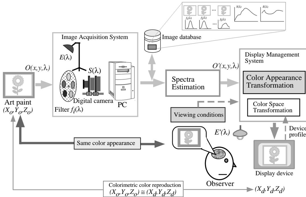
Figure 1. Schematic diagram of proposed color management system.
