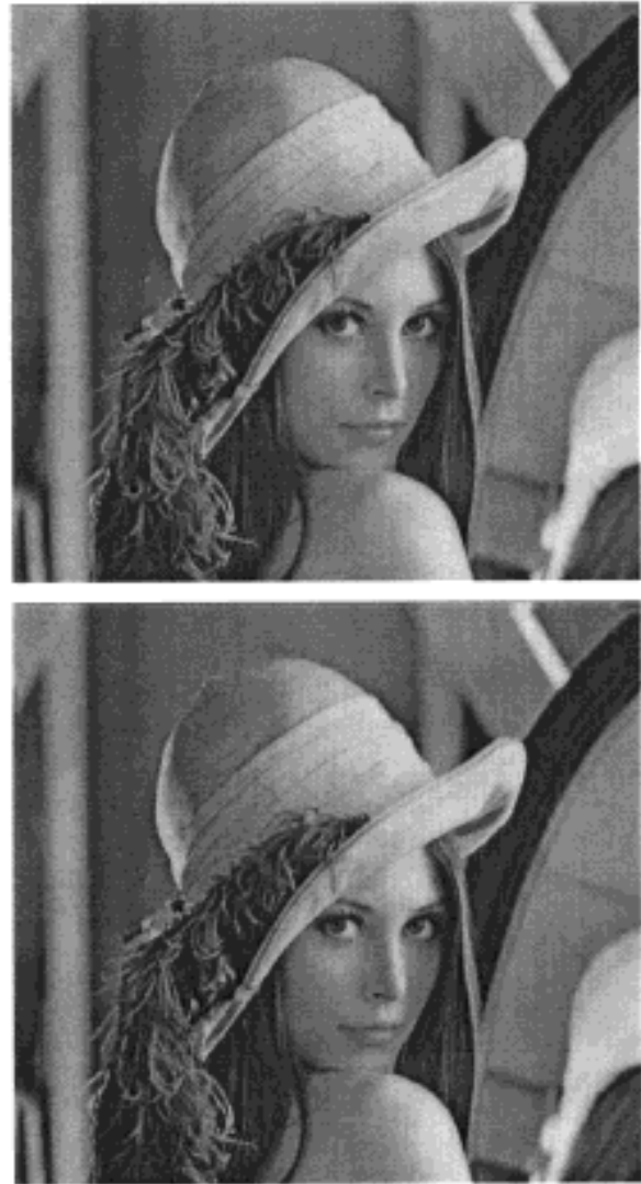
Figure 2 - Original image and image after analysing, pruning, block thresholding and reconstruction. The compression ratio is 1:10.
