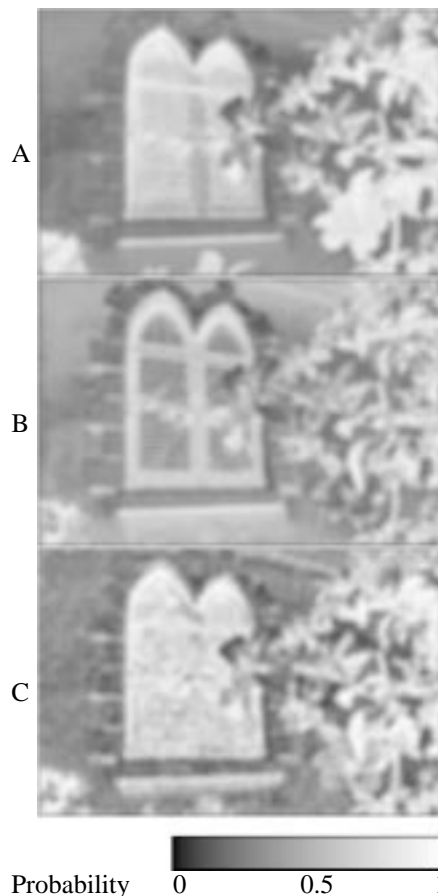
Figure 2: The error maps computed using three different metrics. The three panels show error maps computed using the (A) RMSE, (B) CIELAB, and (C) S-CIELAB methods.
