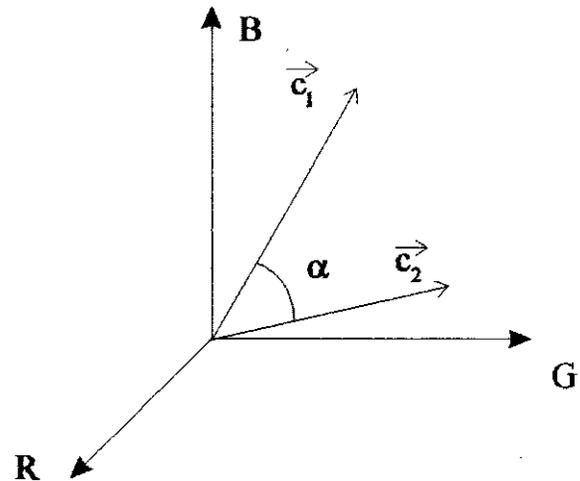
Figure 1. Included angle between two vector colors
