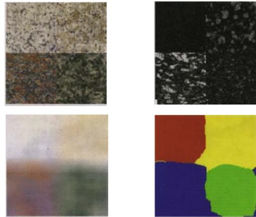
Figure 3. a) the original mosaic b) the "color difference image," e) the "average color image," and d) the classification result.
