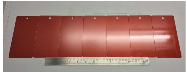
Figure 2. Seven panels with same red metallic basecoat, but covered with different clearcoats varying from matte (left) to high-gloss (right). From left to right, these same clearcoats are referred to as gloss class 1 to 7 in Table 1.
