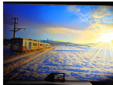
Figure 1. Painting illuminated by two lightings to create a controllable HDR scene up to 10000 \text{ cd/m}^2 and 5000:1 contrast ratio.
