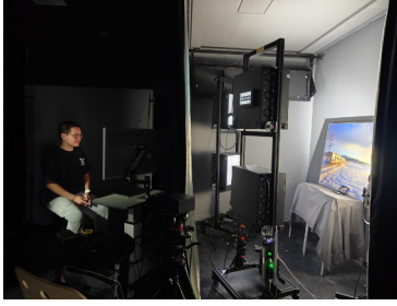
Figure 2. Matching experiment setup: left is a dark room where observer and HDR display, right is lighting system and the painting, the wall in center has a square hole.
