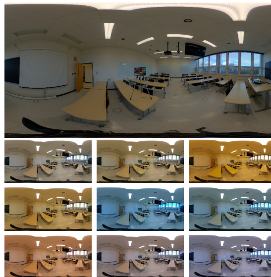
Figure 4. Capturing scenes under different white balance settings. For two different indoor scenes captured in HDR (top, tone-mapped with [19] for display), we also capture a series of JPG images under different white balance settings (bottom), to acquire a rich dataset of realistic color renderings. A color checker is placed in each scene for accurate color calibration.
