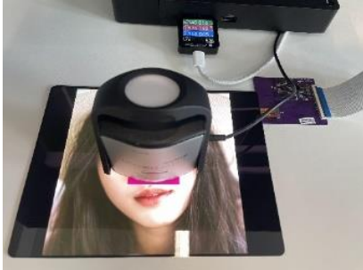
Figure 7: Setup to collect verification ground truth data by capturing the colorimetry of 175 RGB color patches displayed on the top of 19 DXOMARK perceptual images. These colorimetric measurements are compared with the predicted colorimetric values with the results of stage 2 and quantified using CIEDE2000.
