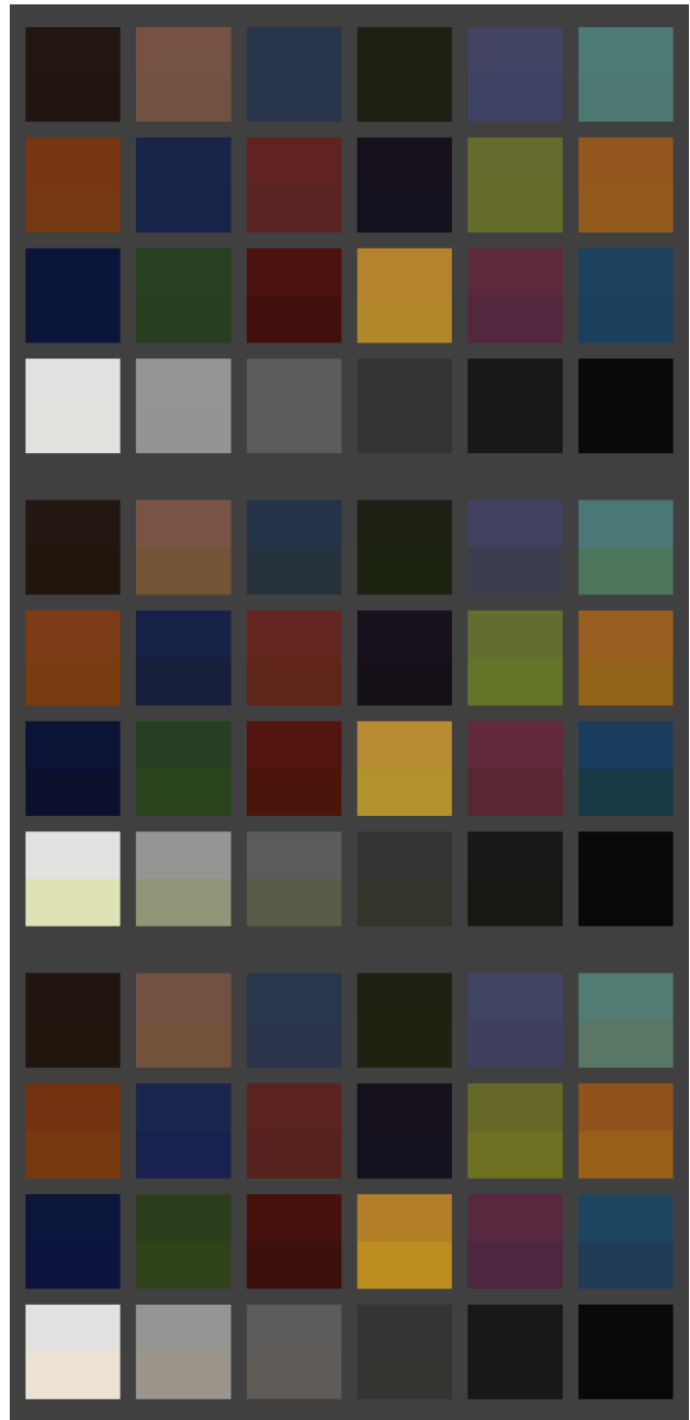
Figure 4. Synthetic Macbeth color checker where the top half of each patch represents the Macbeth patch lit by the reference source, and the bottom by each of the three test sources with an SSI of 63. From top to bottom, the test sources used were SPD1, SPD2, and SPD3. The camera spectral sensitivities used in this illustration were those of Camera 1. These images are not processed for display or printing and are intended to be an illustration of the difference in linear camera response to the test sources vs. the reference source.
