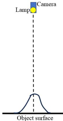
Figure 6. Image capture setup for a glossy flat object surface.
