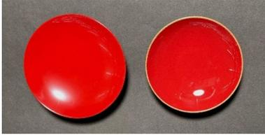
Figure 1. Comparison of two red sake cups. The left cup is a real lacquer cup and the right one is a synthetic plastic cup.
