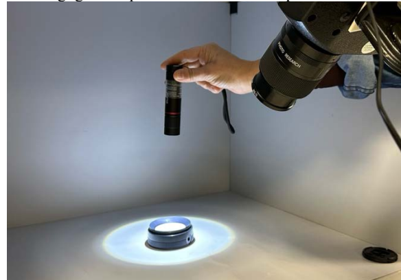
Figure 5: Measurement set-up in a VeriVide viewing booth (with all lights switched off), a calibration tile and the PhotoResearch PR670 telespectroradiometer.
