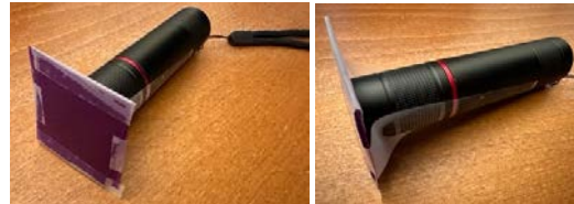
Figure 3. LED torch filtered by stack of five purple gels used in psychophysical experiment.
