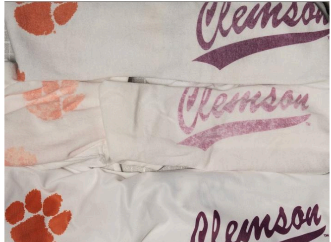
Figure 7. Results for blended (top), cotton (middle), and polyester (bottom) printed with dye sublimation after treatment. The sample in the center shows the instability of this process when printing on 100% cotton textiles.
