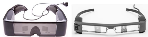
Figure 6. Two AR glasses used in Exp 2 (left: BT-100, right: BT-300).
