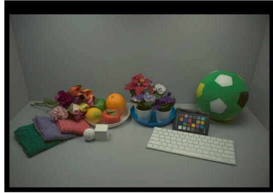
Figure 2 A photograph of the real viewing booth under the illumination of the spectrally tunable LED lighting devices. This photograph is then reproduced with a validated color accuracy on the MR simulator booth (see Figure 5 and description).
