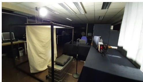
Figure 1: Experiment setup with the car mockup and external illumination simulating the daylight scenario.
