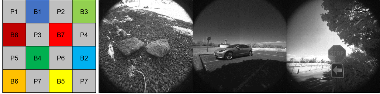
Figure 1. (Left) Pixelated pattern of custom SFA, bands are provided in Table 1. (Right) Examples of raw images acquired by the custom SFA. Vignetting is due to the optical system used for data acquisition (aperture \approx f/4 ) and is corrected during image processing (through a flat-field) after dark signal subtraction. A variety of scenes were used to account for specular reflections, granularity, textures and wide dynamic-range.
