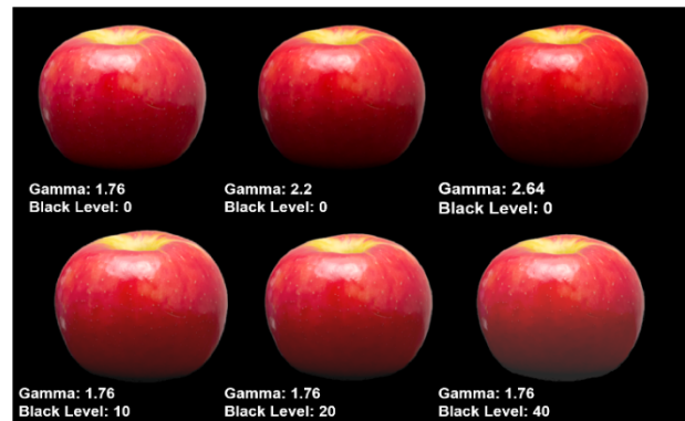
Figure 5. Images of the Apple AR stimulus with six gamma and black level settings on AR display. Gamma changes from top left to top right, and black level changes from bottom left to bottom right.
