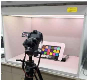
Figure 4. The experimental situation of capturing MCCC in the LED viewing cabinet.
