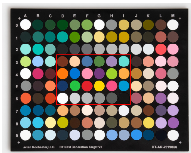
Figure 2: Next Generation Target (NGT) from Avian Rochester ( https://www.avianrochester.com/nextgentarget.php ), LLC. The 24 centered patches are the same as in ColorChecker Classic from X-rite.
