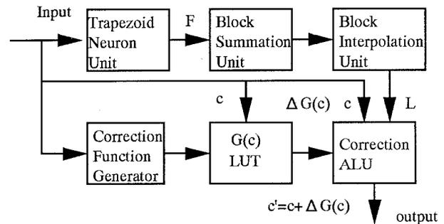
Figure 11. Image correction processor board
