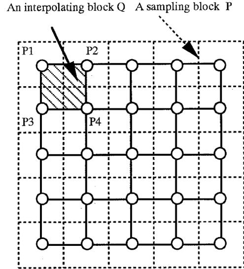
Figure 4. Block summation and interpolation ( $L_{(0,0)}=L_1, L_{(d,0)}=L_2, L_{(0,d)}=L_3$  and  $L_{(d,d)}=L_4$ )
