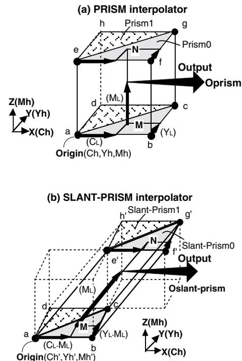
Figure 2. PRISM and SLANT-PRISM interpolator
