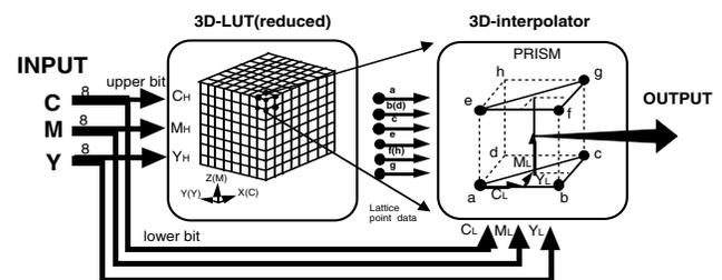
Figure 1. 3D-LUT and interpolation method
