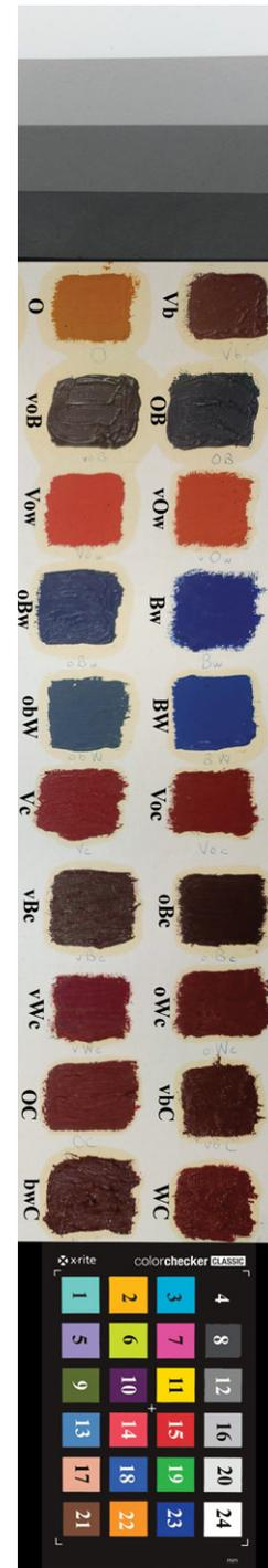
Figure 3. Acquisition arrangement of pigment mockup with the Spectralon<sup>®</sup> multi-step reference target to the left and ColorChecker on the right. Numbering for ColorChecker is added manually here in this figure for reference.
