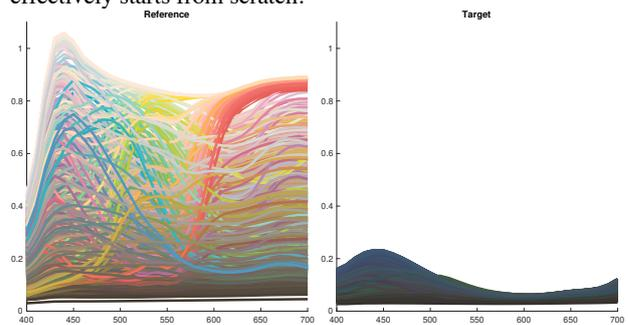
Figure 3. Reflectances of 864 printed patches on canonical, white substrate (left) and on pre-colored, blue substrate (right).
