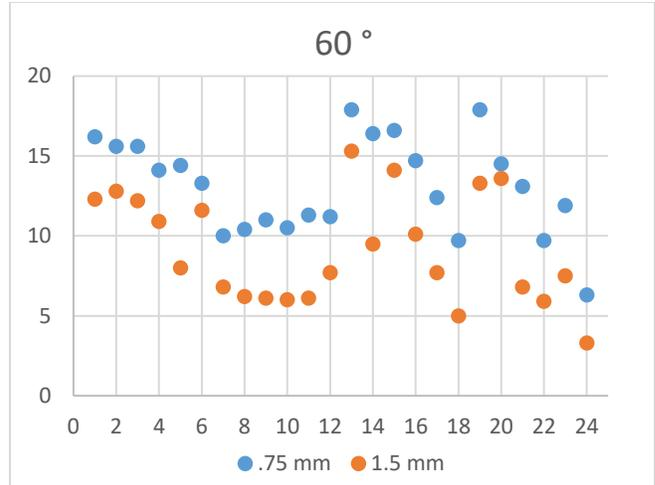
**Fig 3** Specular gloss in GU measured at 60 degrees for maximum height of .75 mm and 1.5 mm
