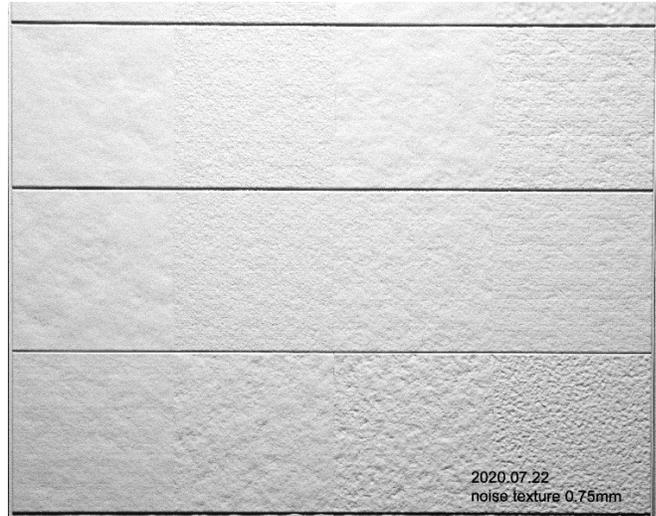
**Fig 2. Inferior section of relief print with maximum height of 0.75 mm based on Perlin noise patches (Fig 10).**
