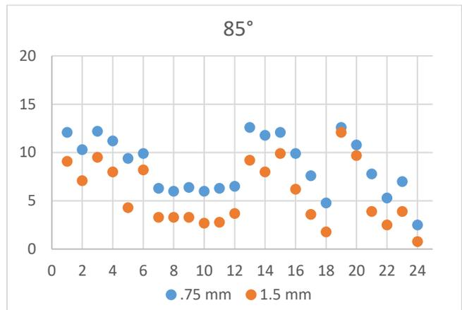
**Fig 4** Specular gloss in GU at measured at 85 degrees for maximum height of .75 mm and 1.5 mm
