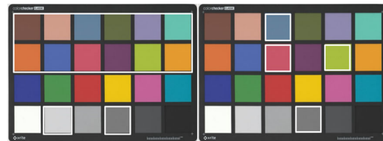
Figure 4. 14 test colours for Display A from X-rite ColorChecker chart (left); and 4 test colours for Displays B, C, and D (right)
