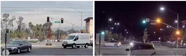
Figure 3. Example images of a crossing from automotive camera, at daytime and nighttime. While the high-contrast TL profiles allow a contour-based state classification in daylight, merely a color-based classification is possible in the dark.
