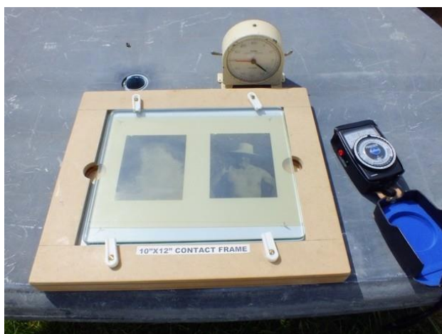
Figure 2. Photopolymer plate with transparent positive film in a contact frame.
