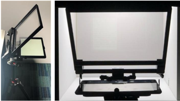
Figure 1. Experimental setup (a) Simulation of Head-up display (b) An example of viewing field (The chin rest is removed for this photograph)
