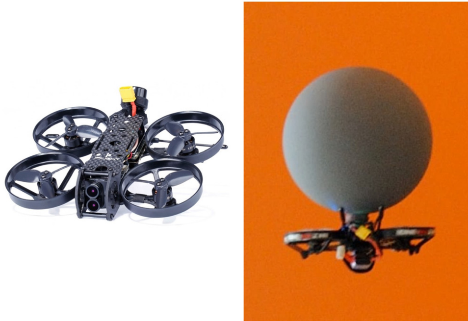
Figure 4. (Left) The CineBee 4K Whoop drone used to carry the gray ball; (right) the gray ball being flown on top of the drone.
