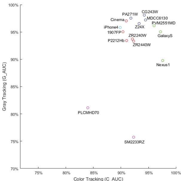
**Figure 4.** The gray tracking (G\_AUC) and color tracking (C\_AUC) of 15 displays. The circles are color-coded by category – green: OLED, blue: professional-grade, red: LCD desktop, cyan: LCD mobile, magenta: special displays
