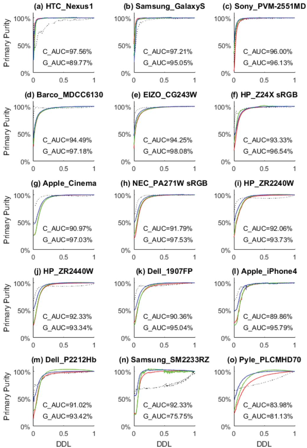
Figure 3. The primary purity and gray purity curves of 15 displays.
