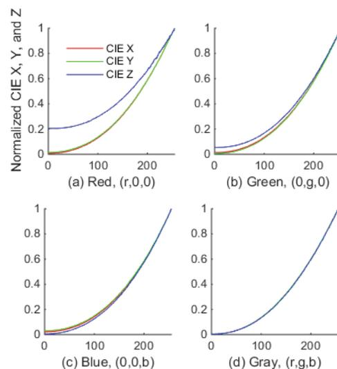
Figure 1. Normalized CIE XYZ measurement results of the red, green, blue, and gray shades of a high-end color medical display (RadiForce R31, Eizo Corporation, Ishikawa, Japan). The overlapped XYZ curves of the gray channel in (d) indicate good gray tracking. The separation between the XYZ curves in the red (a), green (b), and blue (c) channels indicates imperfect color tracking.
