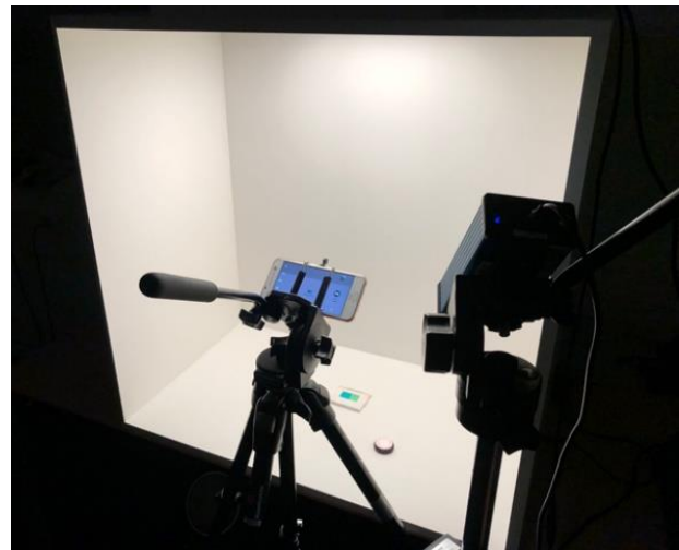
Figure 3. Light box with the melanopic and photopic patch positioned on the bottom. A LEDCube 11-channel LED system on top provided the illumination, images of the patches were recorded by a smartphone (left tripod). The actual spectral power distribution of the illumination was measured by a spectrophotometer (right) pointed at a white calibration patch.
