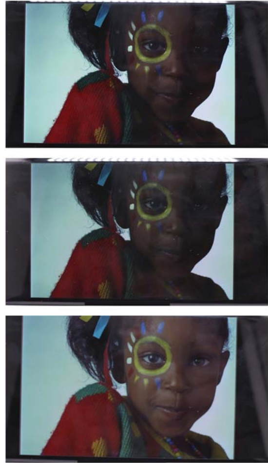
Figure 11. Snapshots of similar OLED displays under ambient light 10K showing the original image (top) at scbr = 100%, original image (middle) at scbr = 60% and processed image at scbr = 60%.
