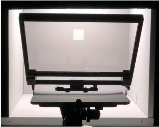
Figure 2 Photograph of the experiment setup. The stimulus was projected from the iPad through the beam splitter.
