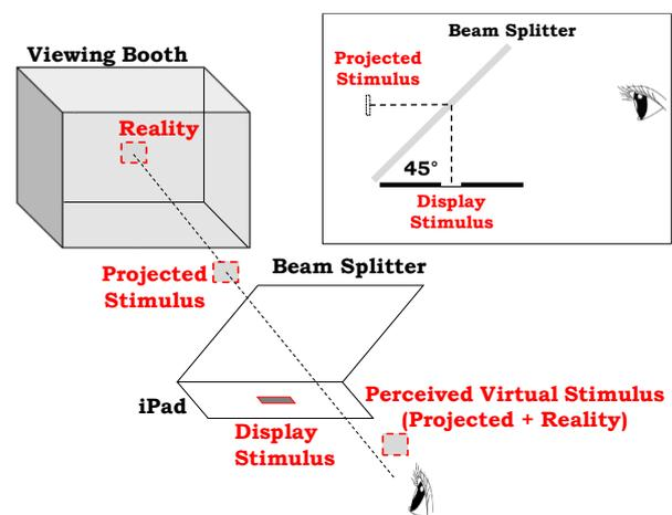
Figure 1 Schematic of the experiment setup. The virtual color was projected by the display colors through the beam splitter. The color perceived by the observers was a blending color of the virtual color and the booth color.
