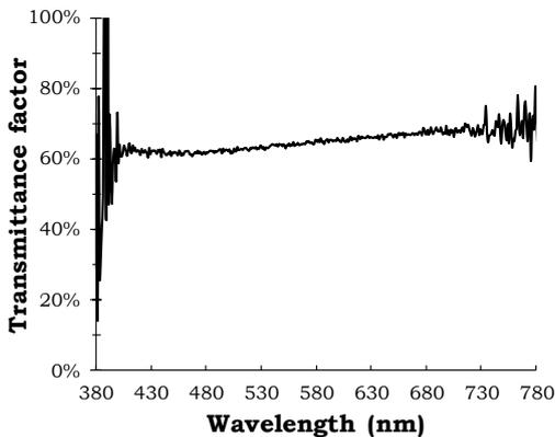
Figure 3 Spectral transmittance distribution of the beam splitter
