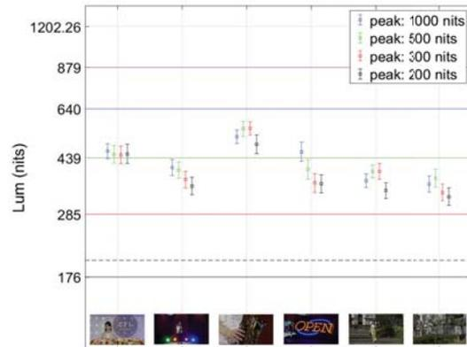
Figure 5: Result of experiment I. Vertical axis is the absolute luminance in log scale. Gray, red, green, blue and magenta solid lines represent the five gray patch levels. Dashed line represents the calibrated 200 nits diffuse white level.
