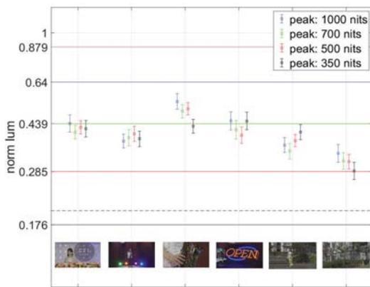
Figure 7: Result of experiment II. Vertical axis is the log scale of normalized luminance level. Gray, red, green, blue and magenta solid lines represent the five gray patch levels. Dash line represents the calibrated diffuse white level, 20% of the peak luminance.
