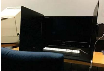
Figure 1: Configuration for experiment I and II, two black matte stands were used to block any possible flare onto the display.
