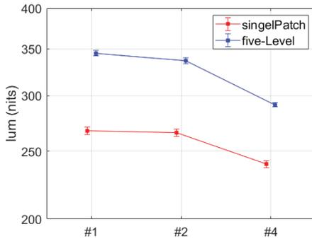
Figure 9: Comparison between result of single-patch adjustment methodology and the five-level methodology for the image#1, #2, and #4.
