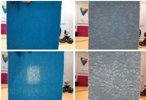
Figure 7. Example of the samples, for which strong directional backlight has statistically significant impact on opacity classification. While they look more opaque in diffuse light conditions (top), they transmit significant amount of light when seen on a strong backlight (bottom).
