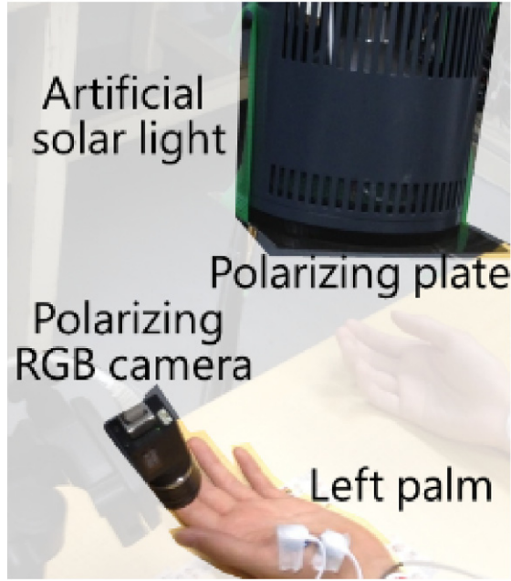
Figure 4. Our experimental setting for constructing a database of images of human skin.
