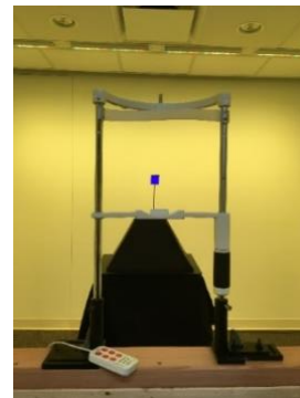
Figure 1. The experiment setup in the light lab, including a chin rest and keypad. In the center of the image is the mirror, subtending about 2 visual degrees, used to display test stimuli.
