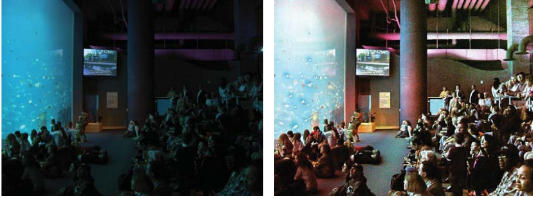
Figure 1: Example of a Retinex artefact. Left: Original Image. Right: Image corrected by using Frankle-McCann Retinex
