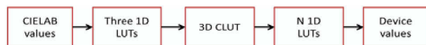
Figure 3. Order of transforms in an inverse tag of a typical v4 ICC profile
