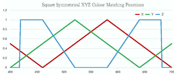
Figure 6 – Three colour matching functions (sensor functions) whose associated colour space has the properties of being complete (no ‘extra-spectral’ colours), computable and regular with respect to saturation.
