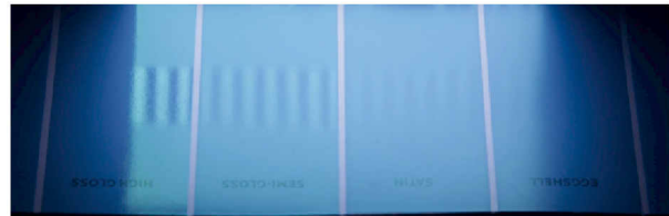
Figure 5. Effects of variations in micro-scale surface roughness on a reflected image. Note the changes in the contrast and sharpness of the reflection as the roughness increases (and gloss declines) from left to right.
