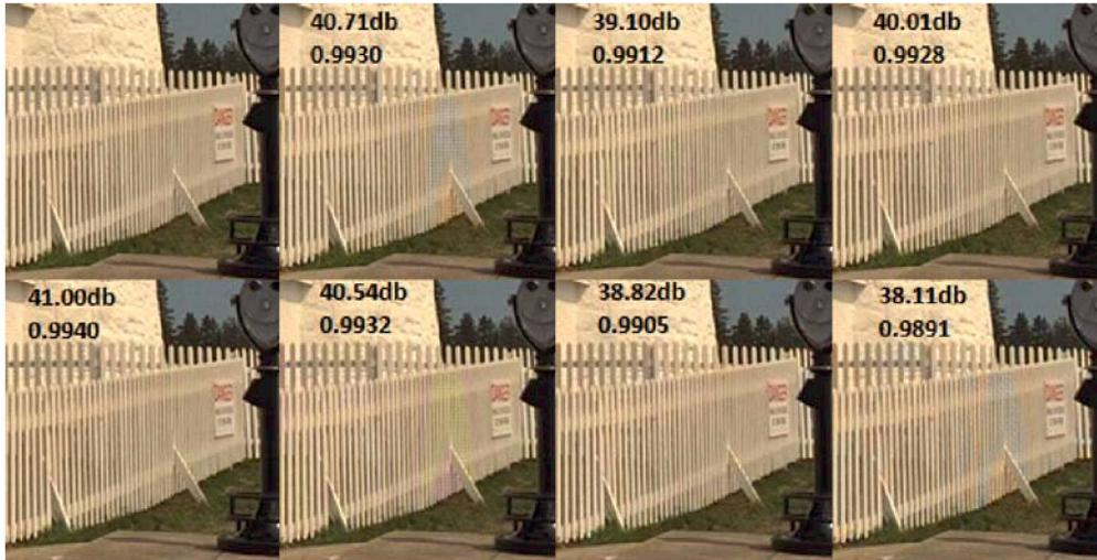
**Figure 3.** Lighthouse Image crop. Demosaiced using our NN method. (Top Row: Left to Right) Original, Bayer, Fuji, CNRS. (Bottom Row: Left to Right) 4x4 # 2, RGBW, Kodak 2.0, Sony RGBW. On the image are presented values of average PSNR ( $\mu$ ) and average SSIM for the entire Kodak database.
