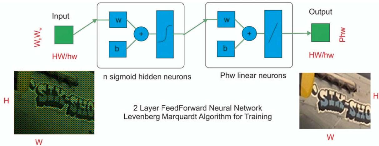
**Figure 1.** Neural Network model used. We used Matlab's Neural Networking toolbox to train our network. A neighborhood window of size  $W_h \times W_w$  is considered around each super-pixel of size  $hw$ . We need to replace  $P$  by  $P_3$  for SFAs.
