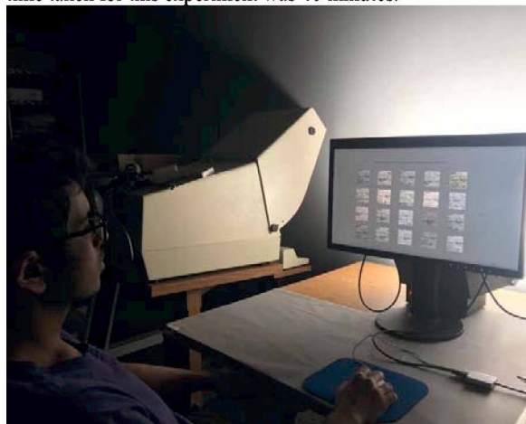
Figure 2: Experimental setup consists of a display showing a GUI consisting of 20 patches for the color quality assessment or 2 anchor images and a test image for the Anchor Scaling. The room lights were switched off and a back light was used.
