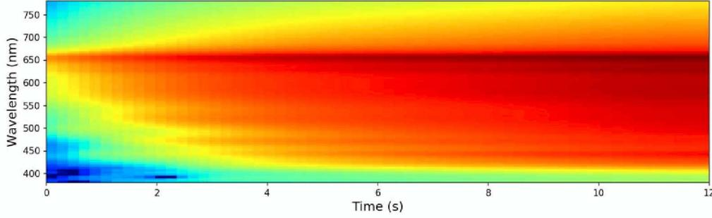
Figure 5. Power-up of an incandescent bulb approximated by an 8-channel luminaire shown as a heat map of spectral power distribution vs. time
