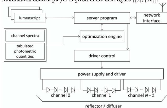
Figure 3. A high-level schematic of an illumination content player
