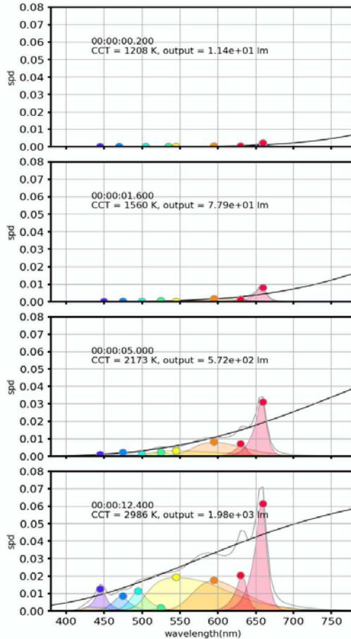
Figure 4. Frames from the incandescent bulb power-up lumenscript compiled for an 8-channel luminaire
