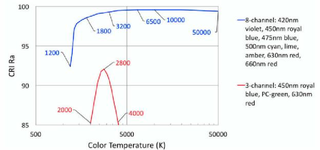
Figure 1. The range of accessible color temperature vs. number of independently controllable channels
