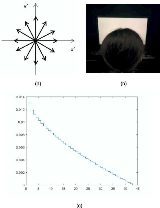
**Figure 1.** Experiment setting. (a) The six color changing directions in CIE 1976  $u'v'$  chromaticity diagram; (b) The experiment situation; (c) A series of color-difference size ( $\Delta u'v'$ ) in CIE 1976  $u'v'$  chromaticity diagram.
