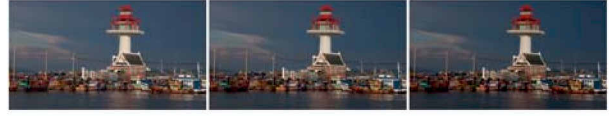
Figure 6. Visual results showing the quality of the power reduction method. Left column: the original image. Middle column: processed image for \gamma = 1 , power saving: 8.01% for scBr = 1 and SSIM = 0.98 . Right column: processed image for \gamma = 2.5 , power saving: 19.4% and SSIM = 0.93 . The savings are for the Google pixel.
